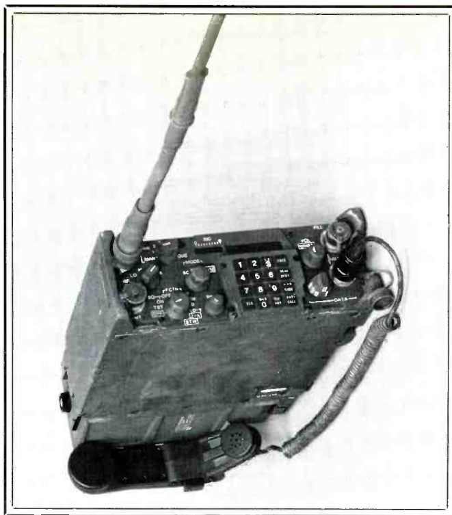
▲ An ITT vehicular short and long range SINCGARS radio.
